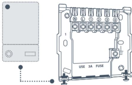
Run cable from the boiler or wiring centre (if required), then continue on to the next section to wire up the backplate.
