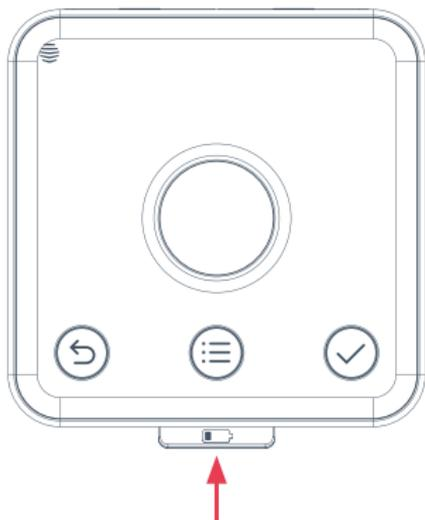
Remove the backplate of the thermostat by pressing the lever at the bottom and pulling away from the front of the device.
