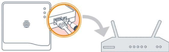
Connect the hub to the household's broadband router using the network cable provided.
