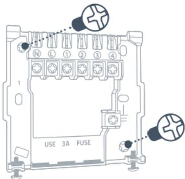
Fix the backplate to the wall with the terminals at the top.
